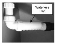
escape into the RV interior. The waterless trap can be unscrewed from the water lines. A label has been placed near the location of the waste valve that reads as follows:
