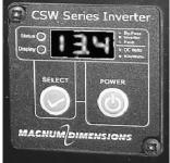
**POWER** button is used to turn the inverter on and off. To
